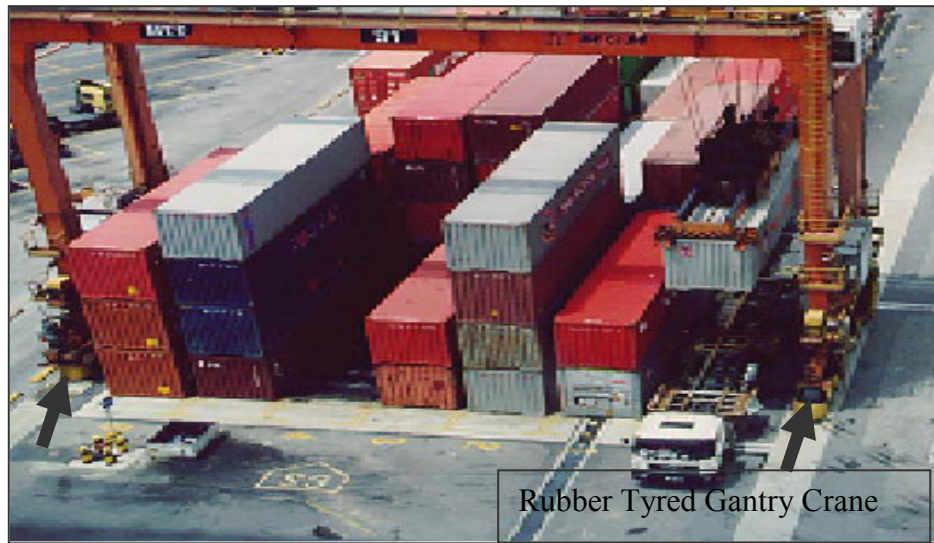
Figure 2-2: An RTGC sits across the width of a block [68]
