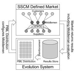
Fig. 3. SMSS feedback loop
